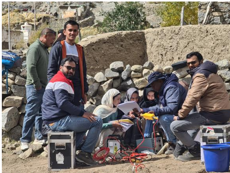
Students learning the multi-electrode resistivity method with NIT Raipur team.
